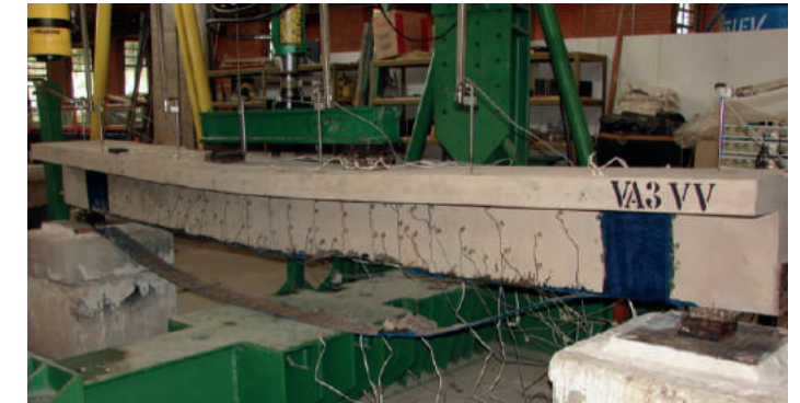
Figure 18. Peeling-off of Glass Fiber Reinforced Polymer (GFRP) laminate and rupture of concrete beam
